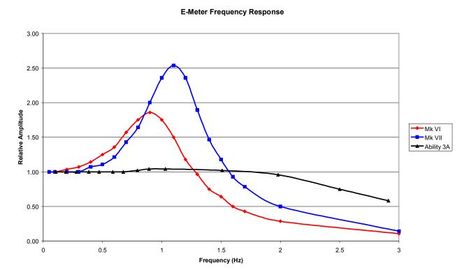
Electronics engineers would normally put such a plot on logarithmic scales. However, for this application, linear scales are more appropriate.
