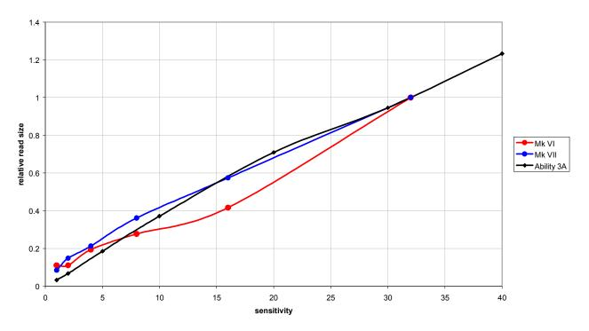
E-Meter Relative Sensitivity Settings (normalised at gain of 32)
